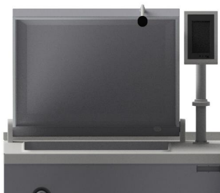
Align the control 90 or 30 with the open cover and screw tight
