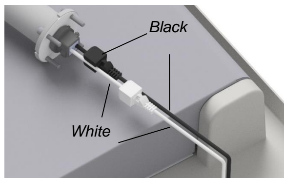
Connect the patch cable - pay attention to the colour!
